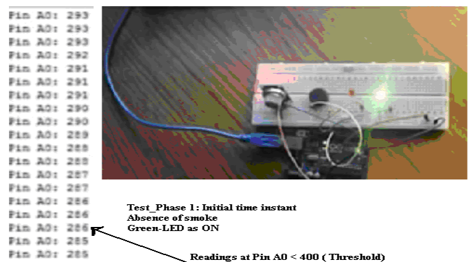
Fig. 15 Test_Phase 1: NO Smoke with GREEN LED
